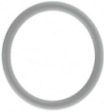
The EPDM O-ring is located within the sensor support and provides additional water ingress protection. The O-ring is typically fitted by FT at the manufacturing stage, but in the event of damage (or general replacement), it can be replaced with care by a technician using tweezers.
